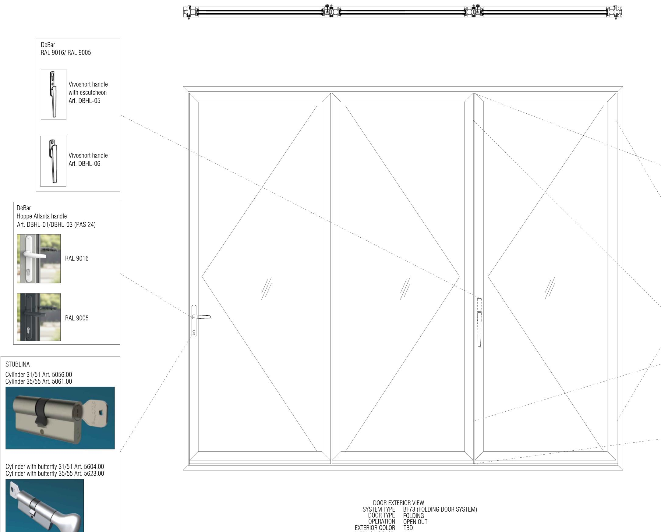
DOOR EXTERIOR VIEW SYSTEM TYPE BF73 (FOLDING DOOR SYSTEM) DOOR TYPE FOLDING OPERATION OPEN OUT EXTERIOR COLOR TBD INTERIOR COLOR TBD GLAZING 1" IGU CLEAR TEMPERED WITH LOW E DeBar Folding door hardware set RAL 9016/ RAL 9005
